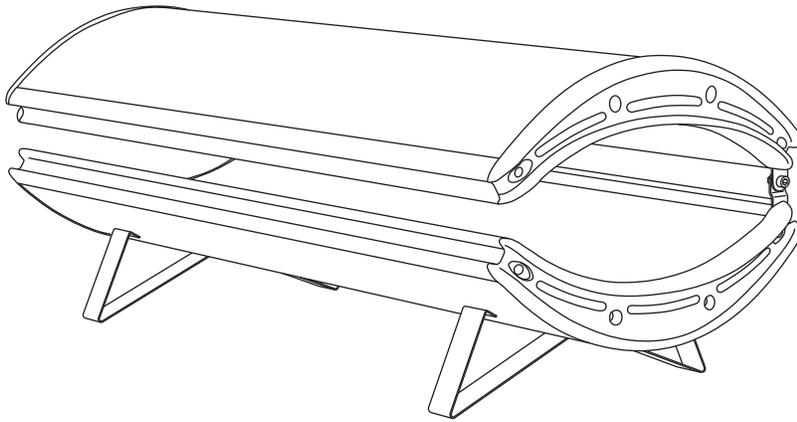
4 Turn the bench over and attach the canopy as shown. Be sure the white Nylon Washer is between the hinges.
